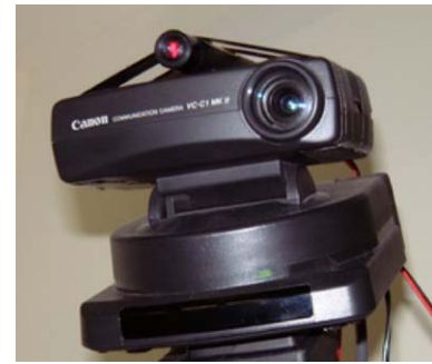
Fig. 2. A laser pointer mounted onto the pan-tilt mechanism of a Canon VC-C1 communication camera.
