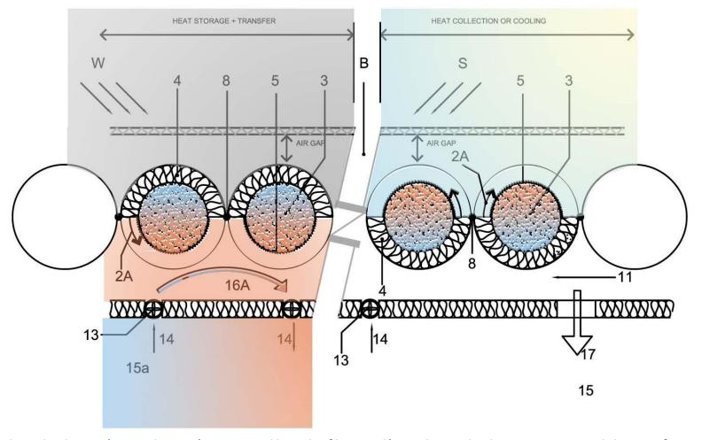
Patent drawing showing on the left portion heat storage and transfer. The insulation is closed (facing outside) so that the collector is radiating heat inside in a way controlled by an inner insulated wall that can be vented or opened to allow heat to the interior in a controlled way.
