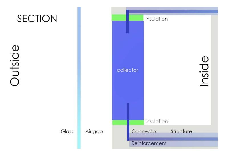
By the morning the collector has been substantially cooled and it can be connected to the reinforcing bars to conduct cool into the thermal mass of the building. Also the collector will radiate cool and reduce air temperatures creating natural air currents.
