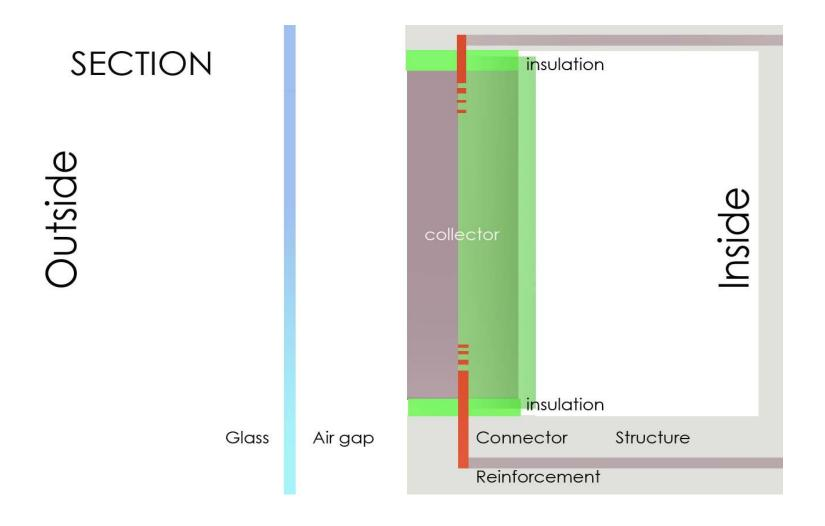
In section, the collector is a heat storage medium insulated from the structure, but can be connected as required to the reinforcing bars to transfer heat or cold to the structure. This is a patented method and overcomes the problem of heat or cold being transferred to the structure when it is not required.
