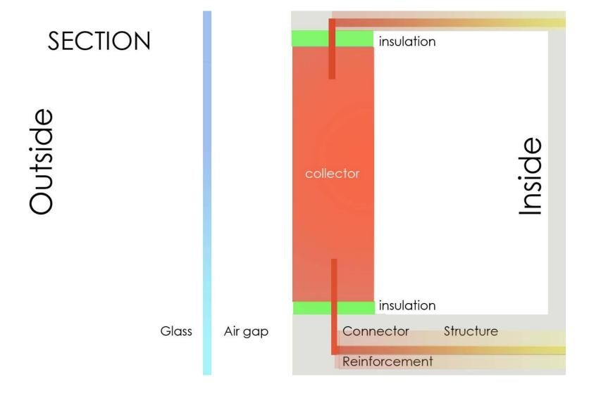
In section the patented solar.fin connector moves to make physical contact between the collector and the steel reinforcement of the slab so that the heat collected is conducted to the general building thermal storage mass
