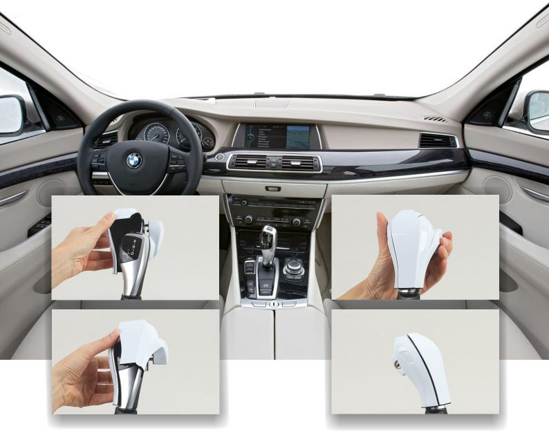
The mechanical security system designed to lock and block the gear lever handle of BMW's automatic transmissions.
