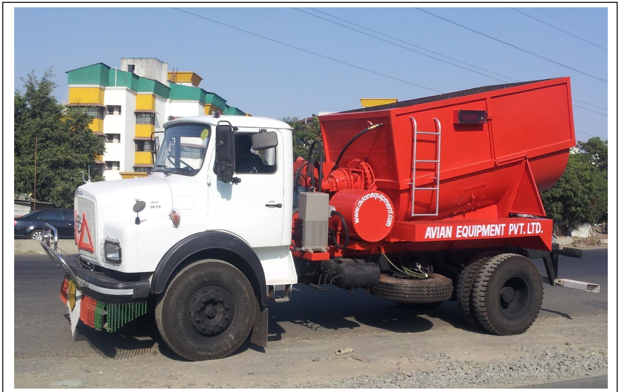
ACTUAL PHOTOGRAPHS OF OM ( SCMD) TRANSIT MIXERS CUM MOBILE BATCHING PLANTS MOUNTED ON VARIOUS TRUCKS ( TATA, ASHOK LEYLAND / EICHER)
