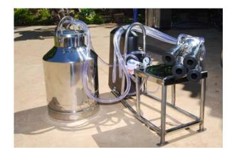
Simple hand operated milking machine has two reciprocating vacuum pump, a handle to operate vacuum pump, a stainless steel machine frame, an air tight stainless steel milk can of 16 liter capacity, a vacuum and pulse regulator with vacuum gauge, 'teat adapter cluster' with a ball valve and connecting plastic pipes.
