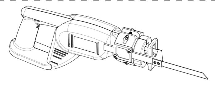
With a simple attachment, a standard center-cut reciprocating saw becomes a flush-cut saw or a power shears
