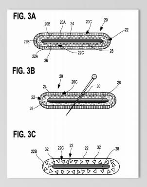
Our Tamper Evident Packaging patent outlines a chemical reaction that warns users if their product packaging has been tampered with by producing a solid substance. (Acts as a warning feature for customers)
