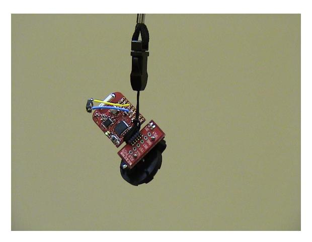
The base unit is under lanyard and always with the users. When it receives RF/wireless signal from the USB device RF transmission unit, the green LED turns on to indicate a corresponding RF/wireless signal (with correct ID number) was received in the last three seconds. The micro-buzzer is OFF at this time.
