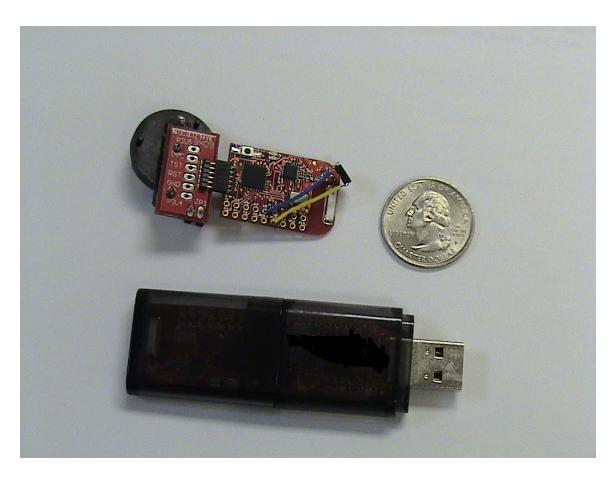
This is a complete set of the base unit and USB device RF transmission unit. The upper side is the base unit with lithium battery. The lower side is the USB device RF transmission unit with a USB type A male connector. (This unit is much bigger than the circuit required due to this is from a general purpose development kit.)
