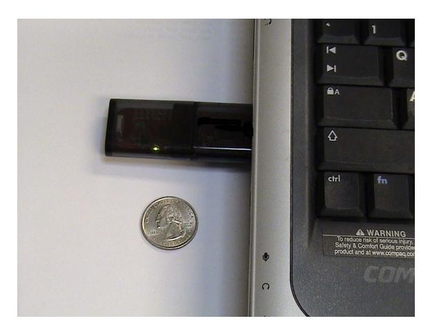
When the USB device RF transmission unit is inserted in a computer, it starts to send RF/wireless signal every second and the green LED lights flash indicate the unit is working properly.
